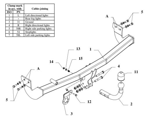
This towbar is designed to assembly in following cars: CITROEN C3 produced since 2002 till 2009, catalogue number P25 and is prepared to tow trailers max total weight 1176 kg and max vertical load 50 kg.
