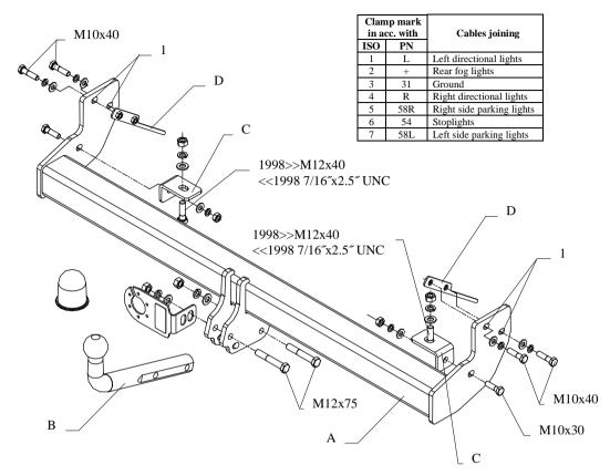
This towing hitch is designed to assembly in following car: **JEEP WRANGLER (TJ),** produced since 08.1996 till 03.2007, catalogue no. **JP 05** and is prepared to tow trailers max total weight up to **2000 kg** and max vertical load **80kg.**
