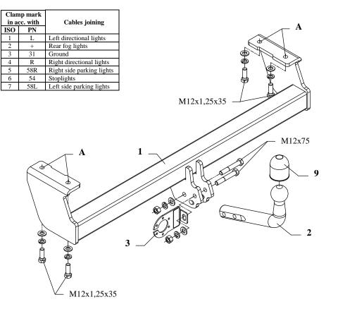
This towbar is designed to assembly in following cars: **SUZUKI GRAND VITARA, 3/5 door,** produced since 09.1998 till 2005 and **SUZUKI GRAND VITARA XL-7** produced since 2001 till 2006, catalogue no. **W08** and is prepared to tow trailers max total weight **1850 kg** and max vertical load **75 kg**.
